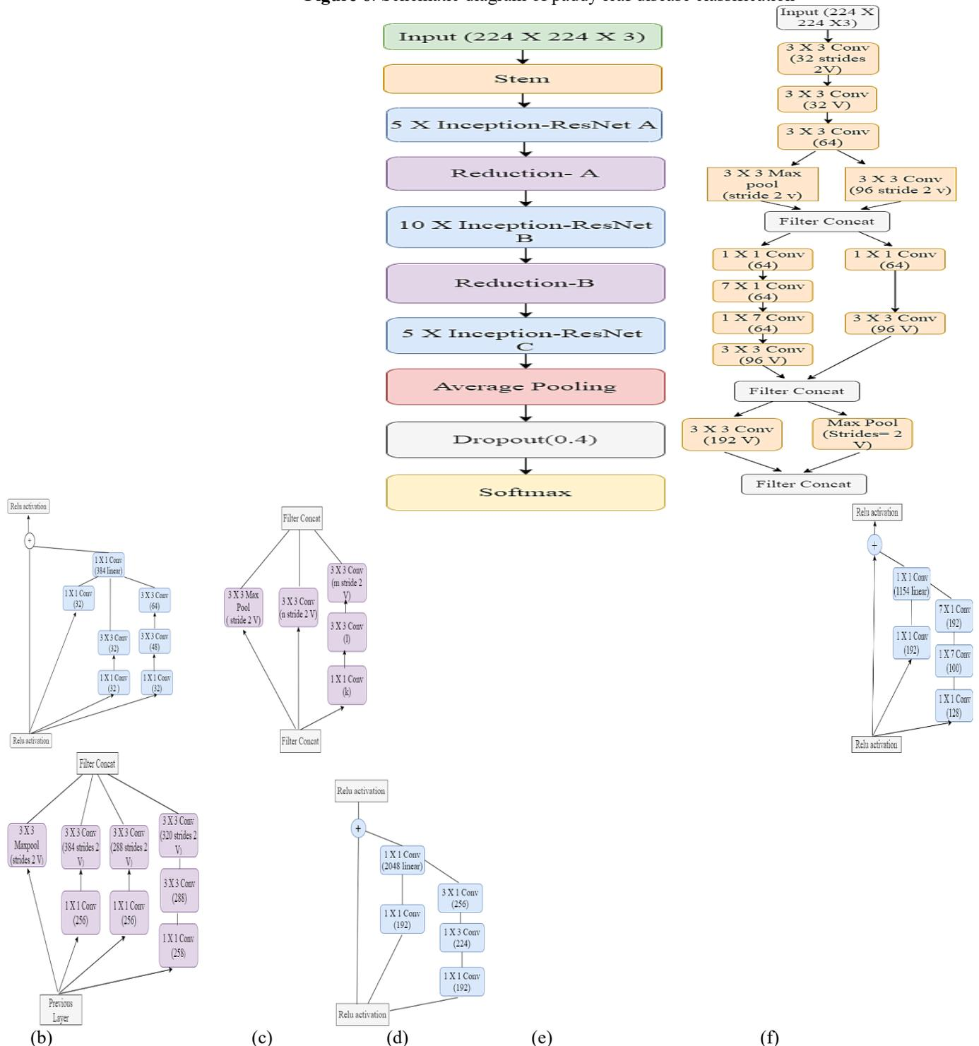
Figure 5. (a) Block structure of Inception- ResNet architecture model (b) Inception resnet A (c) Reduction A (d) Inception ResNet B (e) Reduction B (f) Inception- ResNet C
